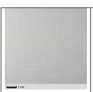
RESIN CONSUMPTION: 63G/M<sup>2</sup> LAMINATE THICKNESS: 0.088 MM, LAMINATE WEIGHT:143G/M<sup>2</sup>
