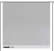
**RESIN CONSUMPTION:** 20G/M<sup>2</sup> LAMINATE THICKNESS: 0.027 MM, LAMINATE WEIGHT: 45 G/M<sup>2</sup>
